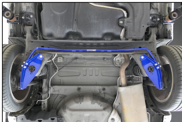
Illustration of installed state 安裝完成示意圖
