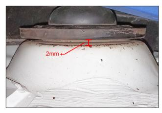
3. Check the distance between strut tower body and upper retaining plates after installation. There should be at lease 2mm clearance for the plates to freely rotate as the wheels turn. 安裝完成後請確認頂端的橡皮固定片及車體避震塔須有至少2mm 的空隙,確保轉向時避震器能自由旋轉。
