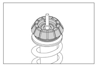
1. Remove the front coilovers from the vehicle to replace the strut mounts. (Spring compressor required)
