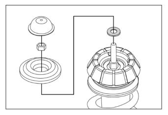
2. Reinstall the coilovers. The supplied washers need to be inserted between the strut mount nuts and upper retaining plates . 將避震器裝回車輛,安裝時請將附件華司裝於避震器座螺帽以及 頂端橡皮固定片之間。
